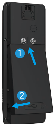
Installation af batteri
